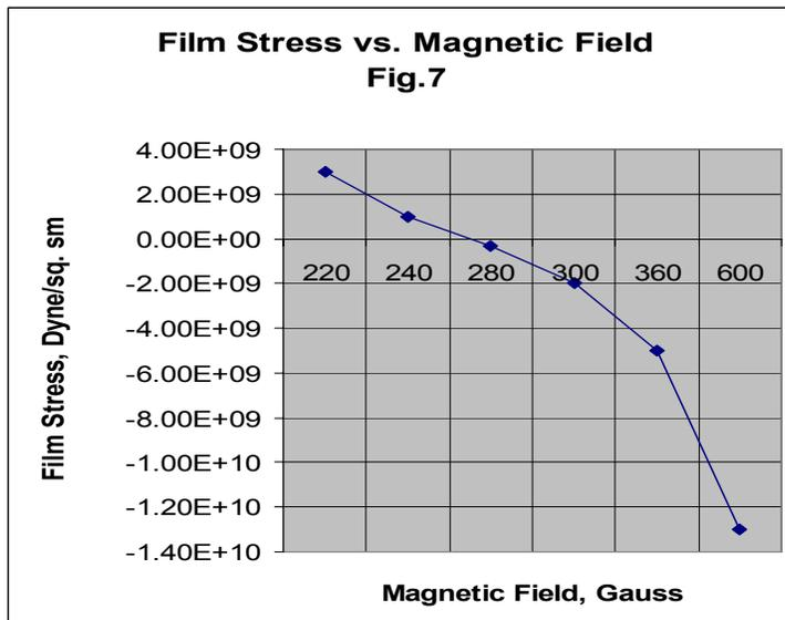
Figure 7 – Film stress as function of the magnetic field strength. The minimum stress occurs at 280 Gauss where it changes from tensile to compressive.
