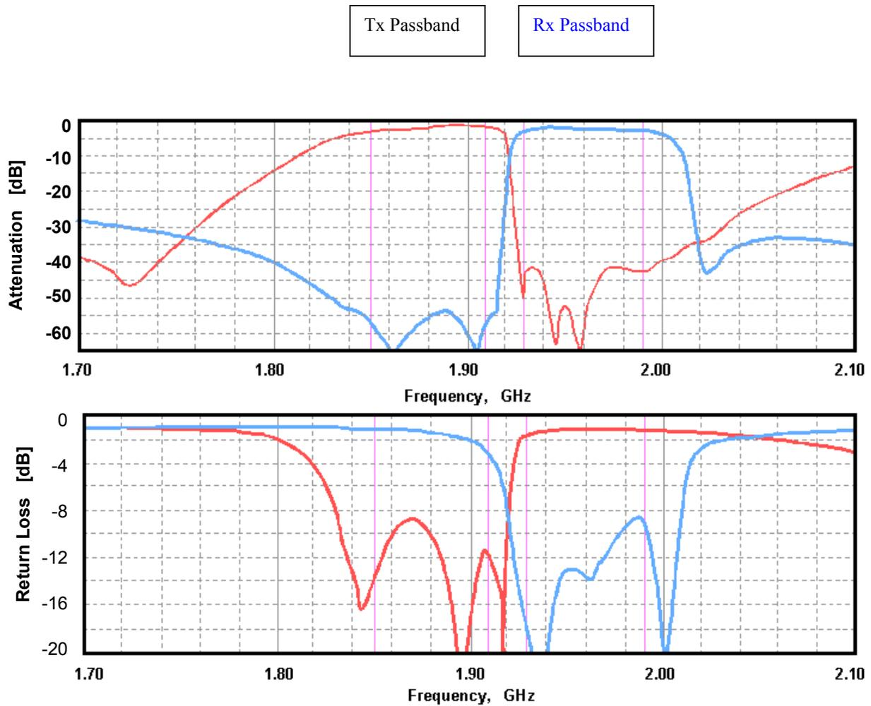
Figure 3 and 4 - Measured performance of an Agilent HPM7903 FBAR duplexer, circa August 2000. Both Attenuation (Insertion Loss) and Return Loss  $|S_{11}|$  at the Rx and Tx ports are shown.
