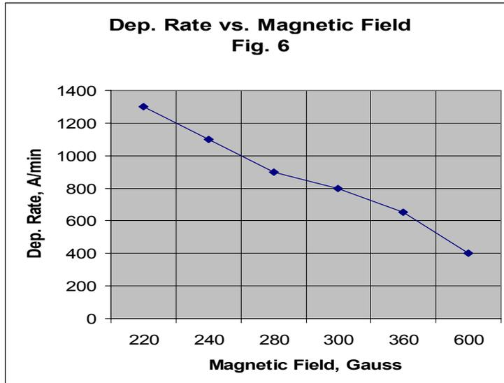
Figure 6 - Deposition rate as function of the magnetic field at the target ring location
