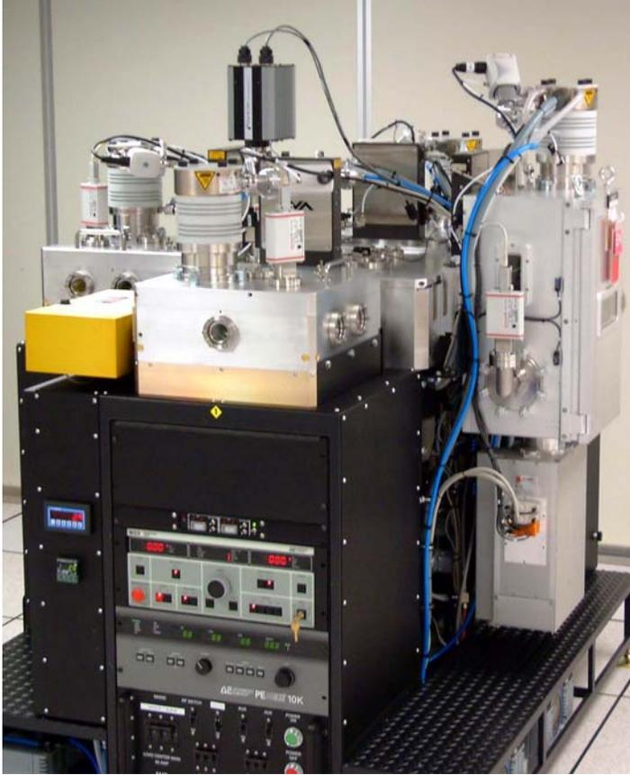
Figure 1 – AMS Custom Cluster Tool for Sputter Deposition.
