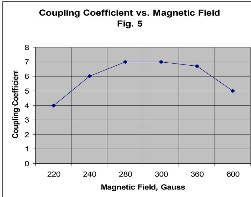
Figure 5 - Film coupling coefficient dependence as a function of the magnetic field strength. Note: for optimum coupling constant  $k_t^2$ , magnetic field  $\sim$  290 Gauss is required.
