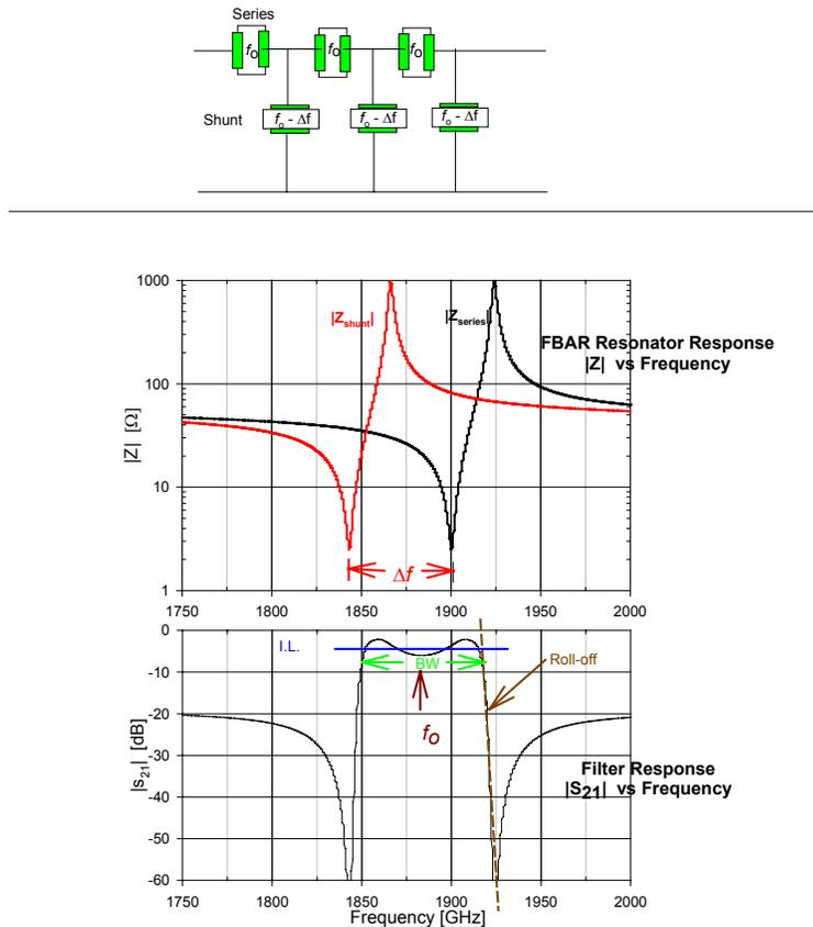
Figure 2 – Illustrating the FBAR resonator ladder filter topology (top panel). The series and shunt resonators exhibit impedance vs. frequency characteristics (middle panel), which produce the filter pass-band response for an RF filter (bottom panel).
