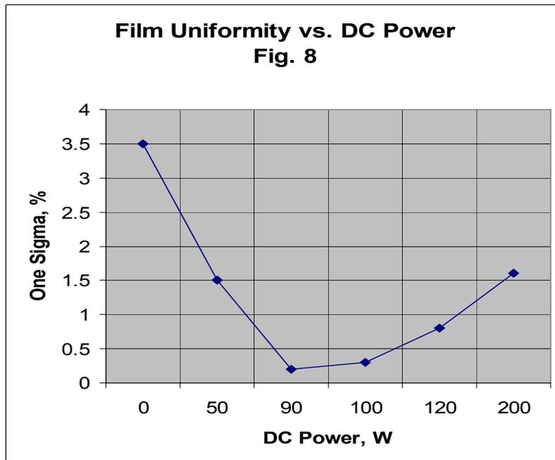
Figure 8– Uniformity of the deposited film for different amounts of power from the secondary DC power supply.
